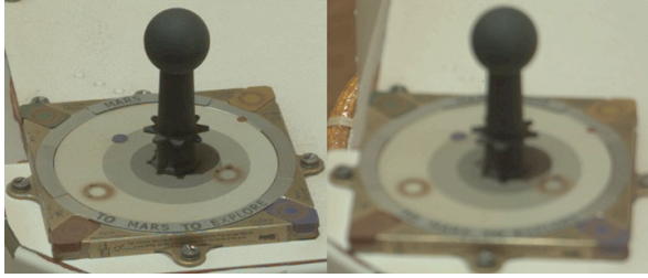
Figure 1. Example Mastcam M-34 (left) and M-100 (right) Filter 0 Bayer RGB images of the Mastcam calibration target [5]. The M-100 image spans ~3x more pixels than the M-34 image; the increased image scale adequately offsets the M-100's inability to focus properly at this close range (1.11 m). Red circular features are airfall dust collecting on strong embedded ring magnets [7].
