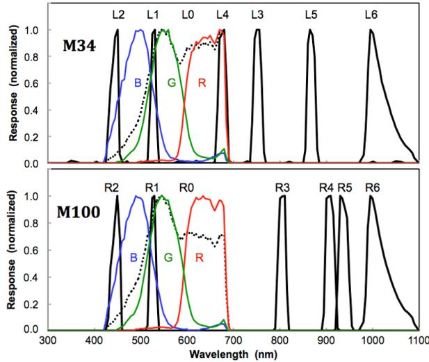
**Figure 2.** Normalized MSL/Mastcam system-level spectral response profiles for the left eye M-34 camera (top panel) and the right eye M-100 camera (bottom panel). When the filter wheel is set to Filter 0 (broadband IR cutoff; dashed profiles shown here), the resulting Bayer filter RGB response profiles are as shown here in red, green, and blue. When the filter wheel is set to a nonzero number, however, the response profiles of the Bayer filters are as shown in [5].
