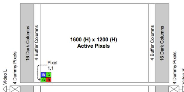
**Figure 1.** Simplified schematic of the Kodak KAI-2020 interline transfer CCD used in the MSL Mastcams [6], along with a graphical representation of each of the 2x2 Bayer RGB filter unit cells bonded directly onto the CCD's active pixels.
