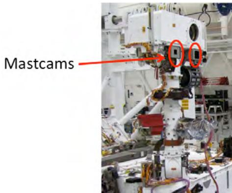
**Figure 4.** Location of the Mastcams on the MSL Remote Sensing Mast (RSM). The Mastcam-Z cameras will be mounted in a similar location on the Mars 2020 rover. Photo credit: NASA/JPL
