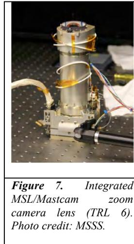
Figure 7. Integrated MSL/Mastcam zoom camera lens (TRL 6). Photo credit: MSSS.
