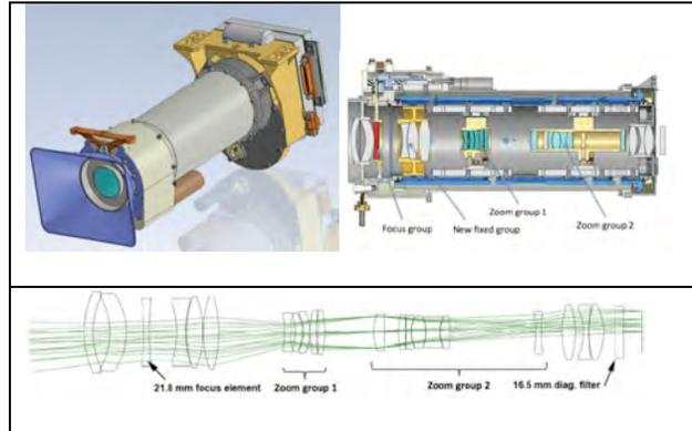
Figure 6. Mastcam-Z camera head (top left, isometric view, top right, cross section). Bottom, optical ray-trace diagram. Credit: MSSS.
