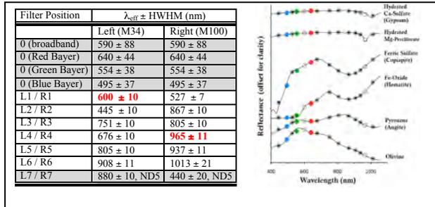
Table 2. Left: Mastcam-Z multispectral filter band centers and widths, with proposed new filters listed in red. Right: Lab spectra [9,10] of hydrated minerals convolved to the Mastcam-Z narrowband and RGB filters (open circles are Mastcam-Z filters, solid circles are MSL Mastcam filters).
